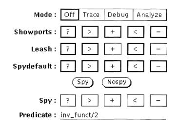
The first item sets the debugger mode. The debugger can be switched off, in which case the engine executes queries in normal mode. It can be in either trace or debug mode, which is the same as when the builtin predicates **trace/0** or **debug/0** are invoked. The last mode is analyze, which is the mode that results from calling the builtin **keeptrace/0**.
