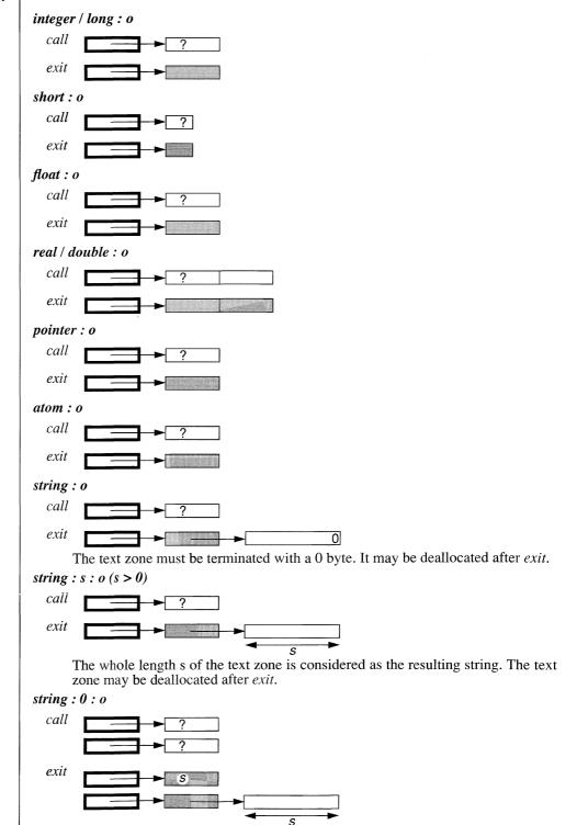
The external routine has to indicate the length of the text zone at *exit*. The text zone may be deallocated after *exit*.
