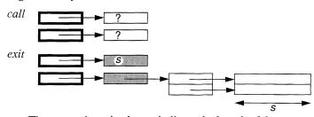
The external routine has to indicate the length of the text zones at *exit*. The pointer array and text zones may be deallocated after *exit*.
