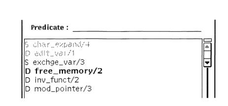
In the list of selected predicates, the class a predicate belongs to is indicated by the corresponding abbreviation in the left column. Hidden predicates are displayed in grayedout font. Debug coded predicates are indicated by using a bold font.
