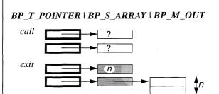
The array is long-term memory and must be freed when no longer needed. *Remark*: This parameter has a *size* descriptor argument, immediately preceding the value argument.
