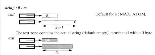
The external routine has to indicate the length of the text zone at *exit*. And  $s_2 \le s_1$ . The whole length  $s_2$  of the text zone is considered as the resulting string.
