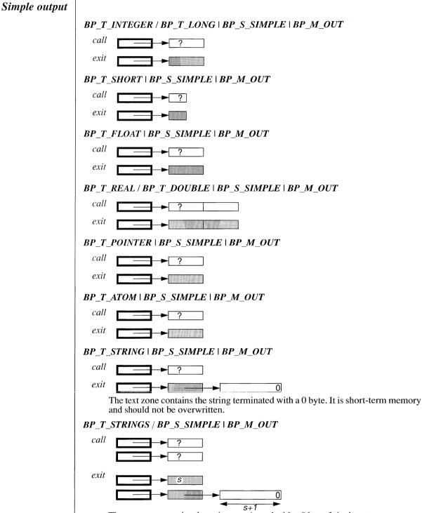
The text zone contains the string terminated with a 0 byte. It is short-term memory and should not be overwritten.
