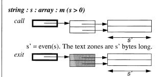
The whole length s of the text zones are considered as the resulting strings. The text zones may be deallocated after *exit*. *Remark* : The text zones at *exit* are not necessarily the same as those at *call*.
