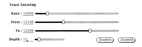
The arguments that will be used, are retrieved from the sliders. The **From** and **To** sliders give the first and second argument for **zoomln/2**. The **From** and **Depth** sliders are used for the arguments of **zoomld/2**.
