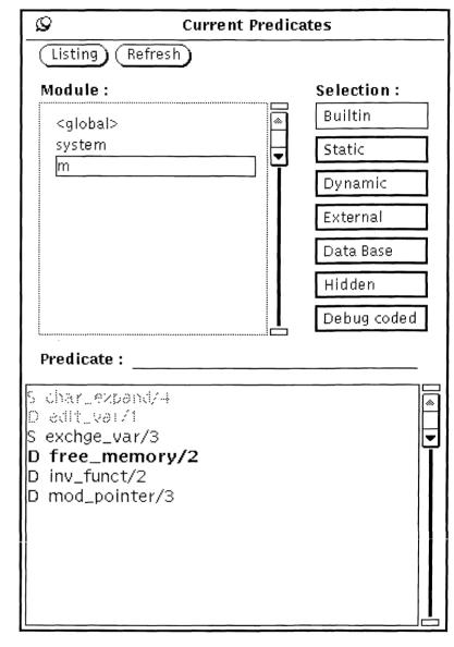
The window contains two selection fields: one for the module and one for the predicate classes. The lower part of the window displays the list of selected predicates.
