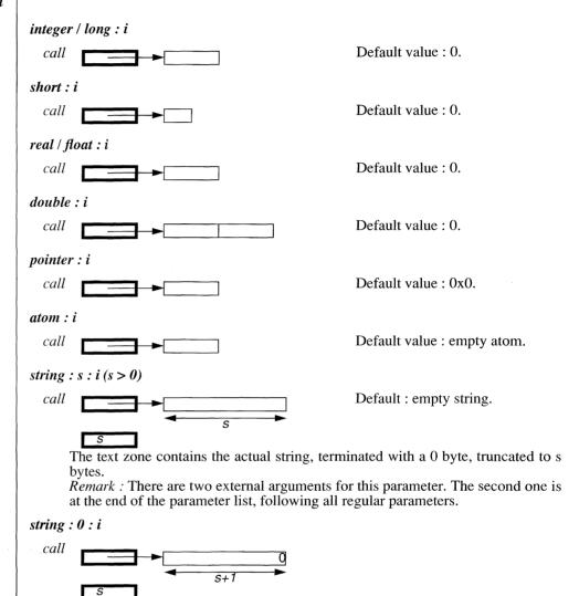
The text zone contains the actual string (default empty), terminated with a 0 byte. *Remark*: There are two external arguments for this parameter. The second one is at the end of the parameter list, following all regular parameters.
